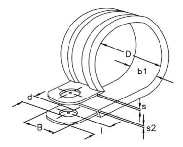
$\begin{array}{lll} b1 & = 15.0 \\ d & = 6.4 \\ Diameter D = 41 \\ I & = 6 \\ s & = 0.8 \\ s2 & = 1.2 \\ Width B & = 12 \\ \end{array}$
